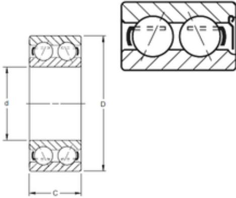
5208WD Bearing 2D drawings and 3D CAD models
